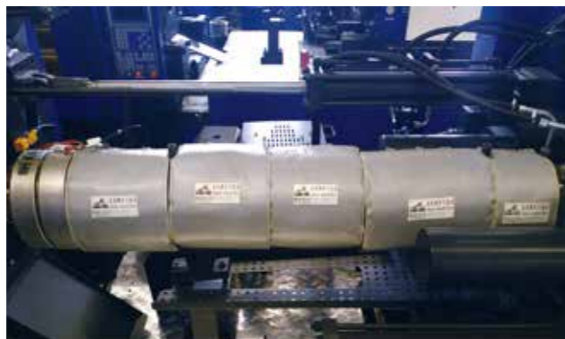
Increased power of the heating ring with optional nanometre energy-saving ring
